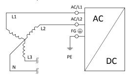
Using a fuse or a circuit break to protect the AC/L2 input is suggested. The AC/L2 input is internally non-protected.
